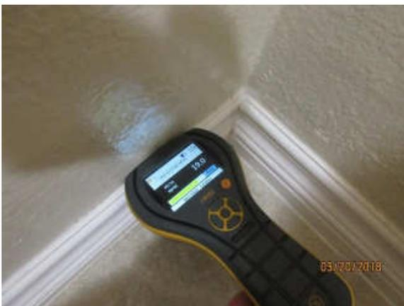
*Elevated moisture readings on east wall*
