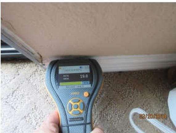
*Elevated moisture readings on wall next to slider*
