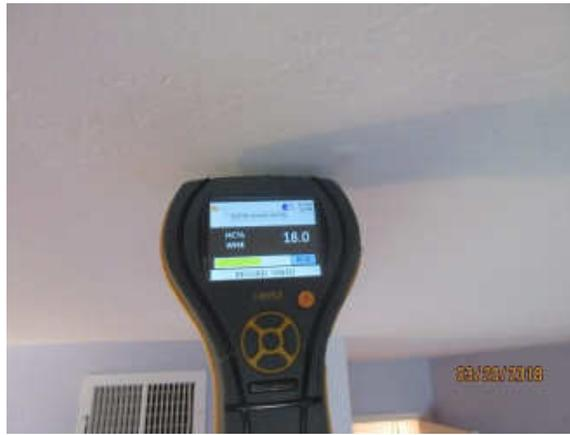
*Elevated moisture readings on ceiling near center of room*
