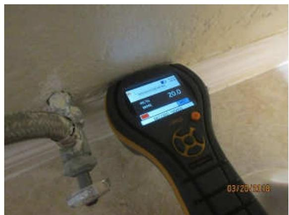
*Elevated moisture readings on south wall*
